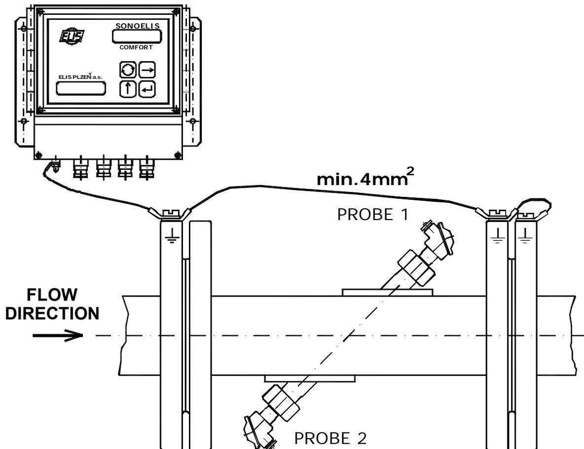
Fig. 14 - Earthing of the electronic unit and flow-meter sensor
