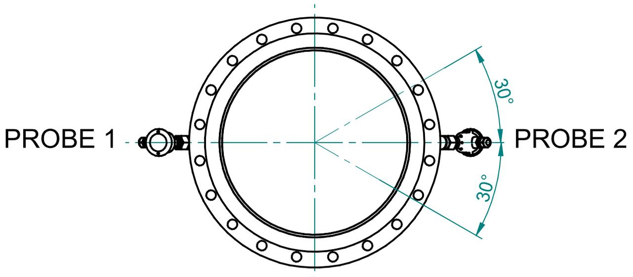
Fig. 13a - Permitted range of one-beam sensor rotation with respect to its longitudinal axis (SE4015)
