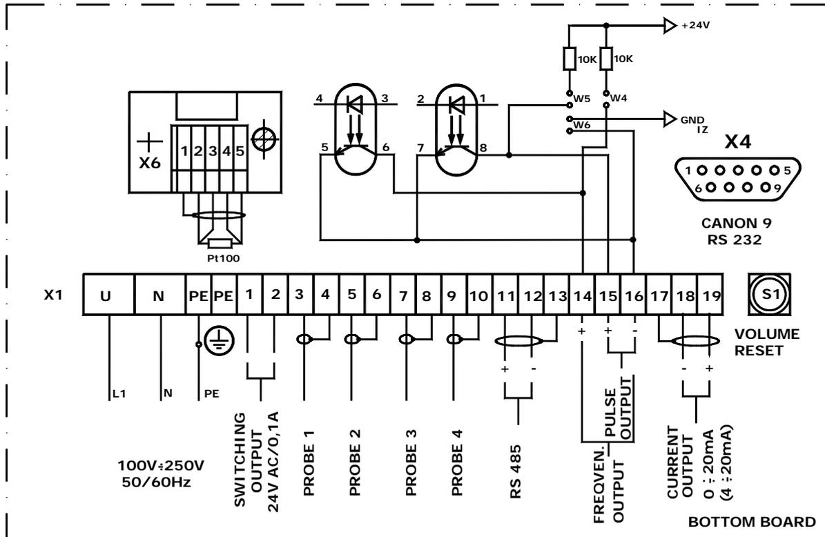
Fig. 15b - Schematic drawing of connections to the SE4025 ultrasonic flow meter
