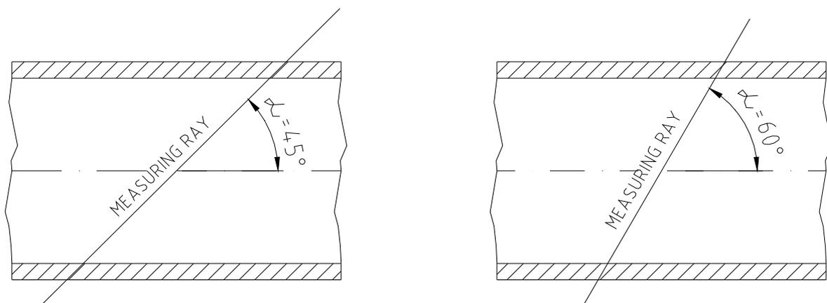
Fig.1 - The ultrasonic ray angle with respect to the piping axis
