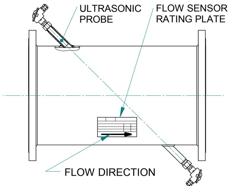
Fig. 4 - Ultrasonic sensor - description
