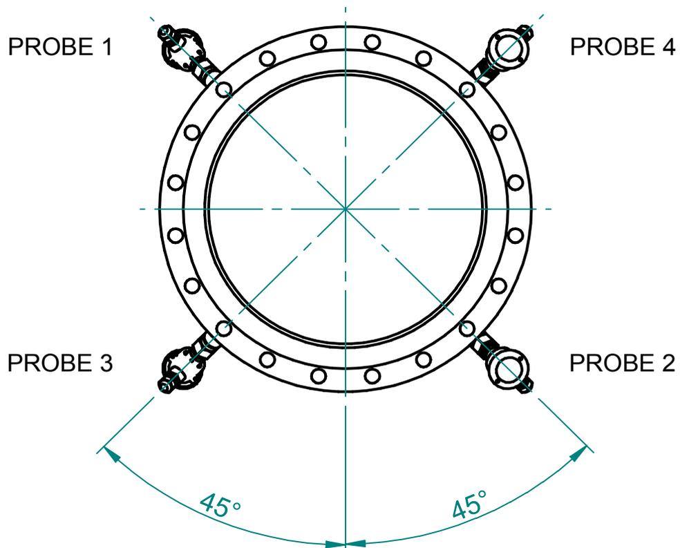
Obr. 13b - Angel between probes planes and vertical plane at double-beam sensor (SE4025)
