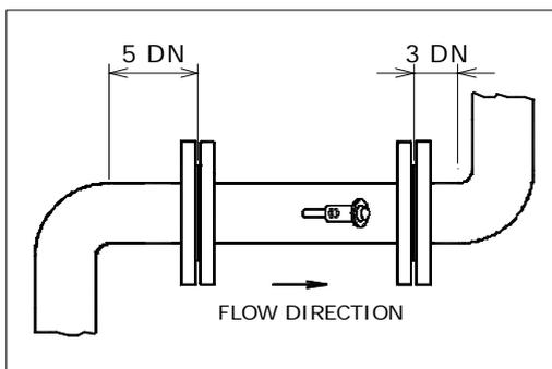
Fig. 7 - Minimum lengths of straight piping sections the input side of closing valve
