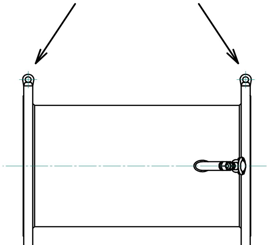
Fig. 6 - Correct grip on the meter sensor
