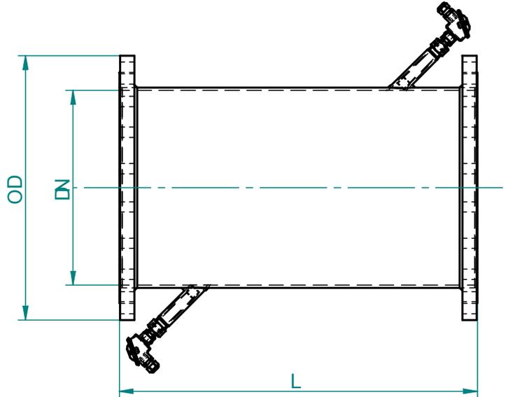
Fig.2 - Dimensional sketch of the meter sensor
