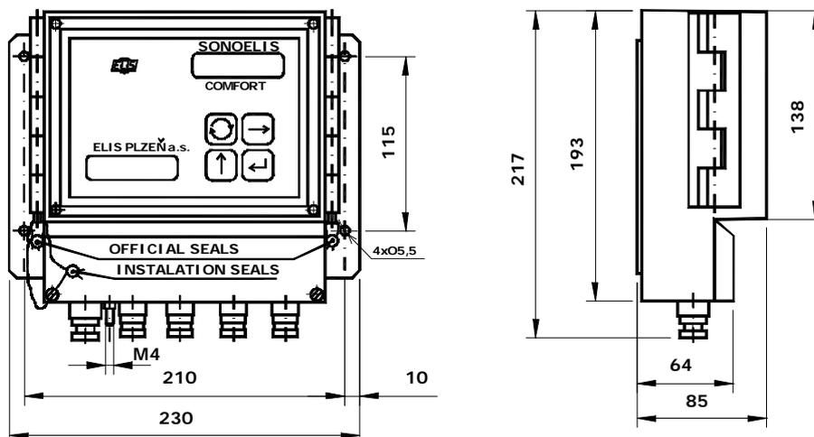
Fig. 3 - Dimensional sketch of the electronic unit box
