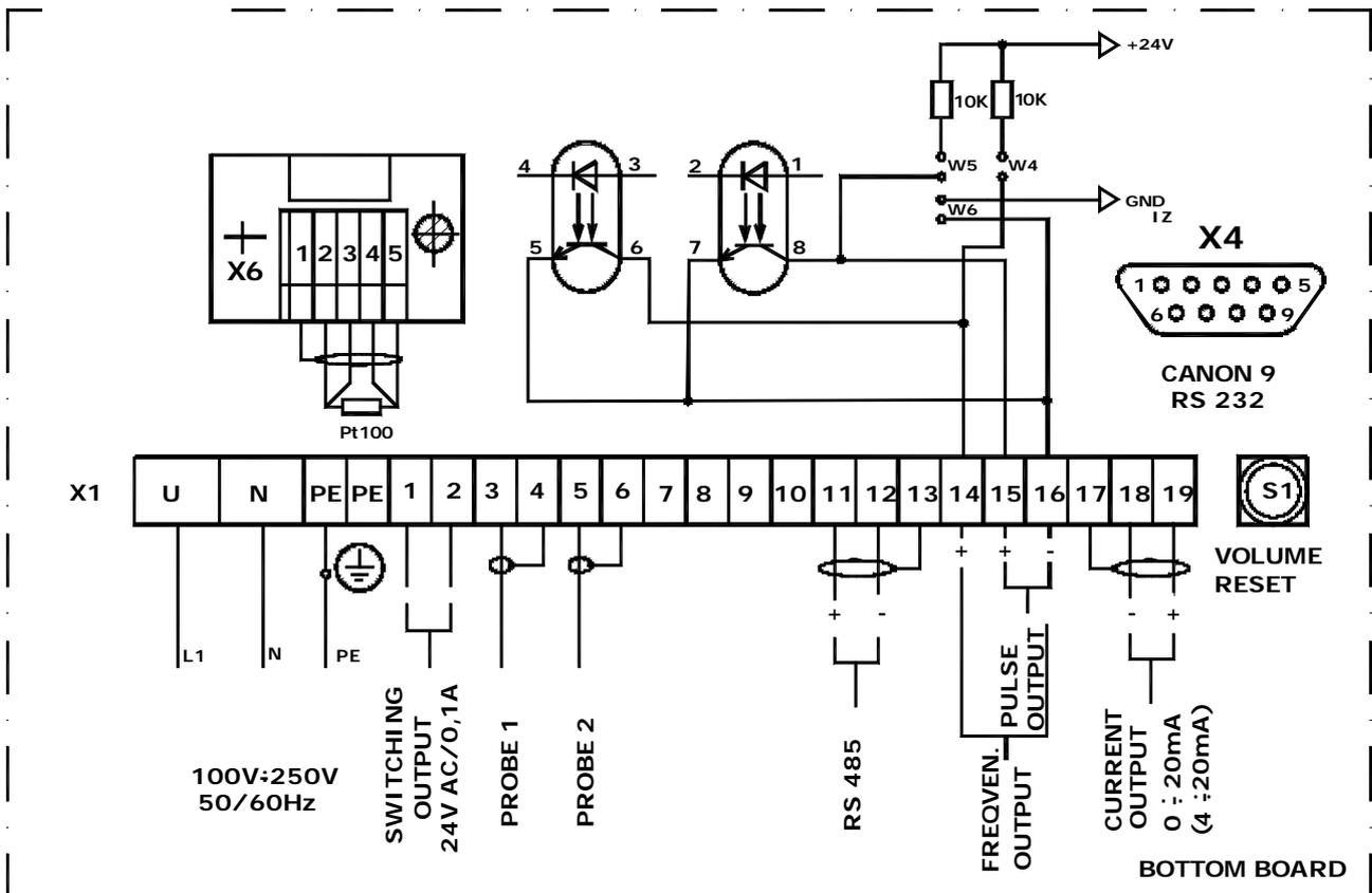
Fig. 15a - Schematic drawing of connections to the SE4015 ultrasonic flow meter
