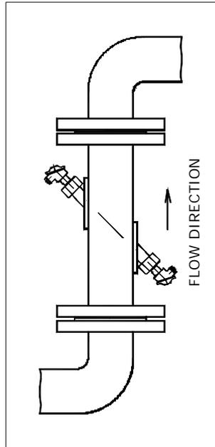
Fig. 11 - Sensor fitted into a vertical piping section
