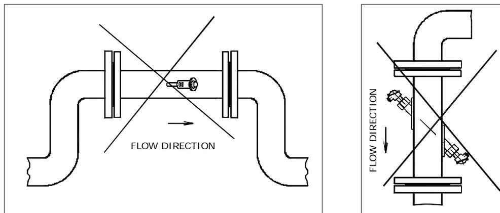
Fig. 12 - Examples of incorrect sensor placement
