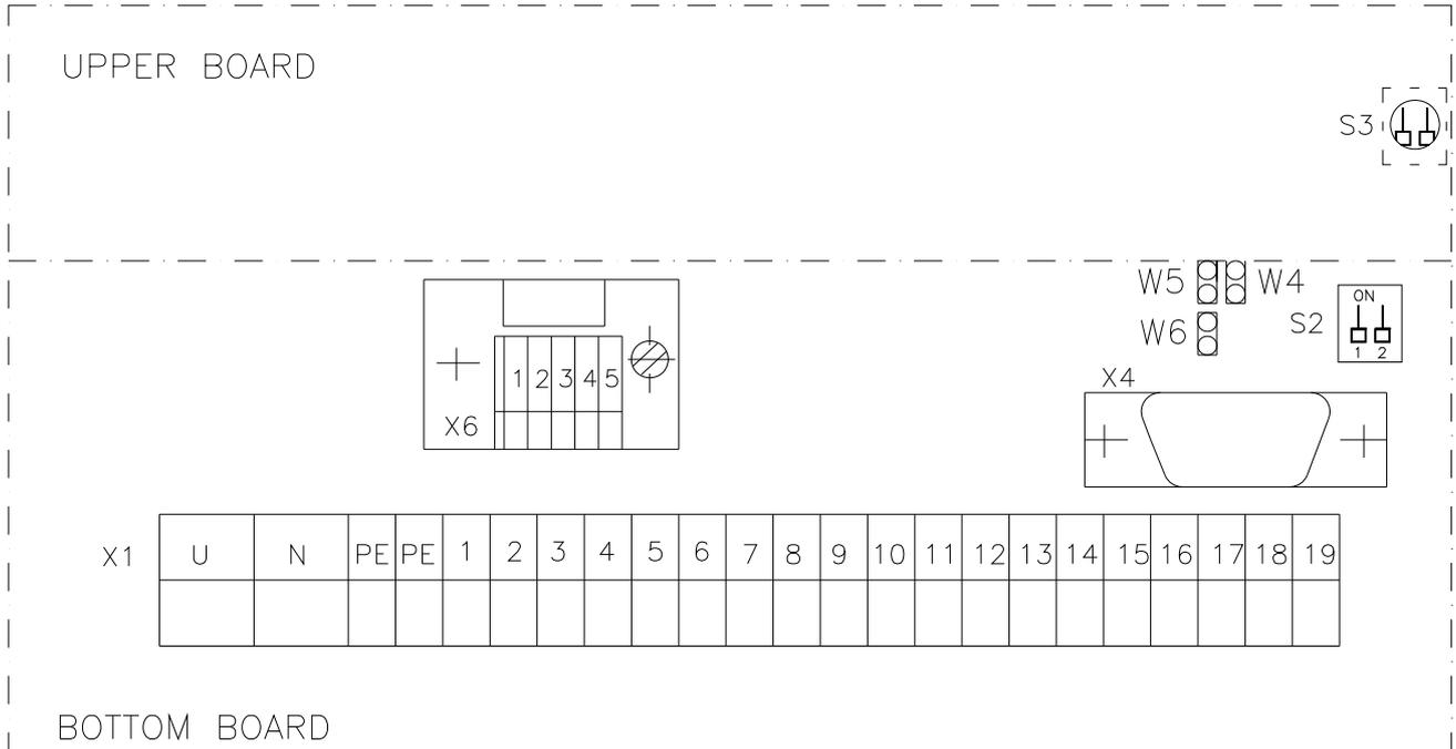
Fig. 16 - Location of switches S2 and S3
